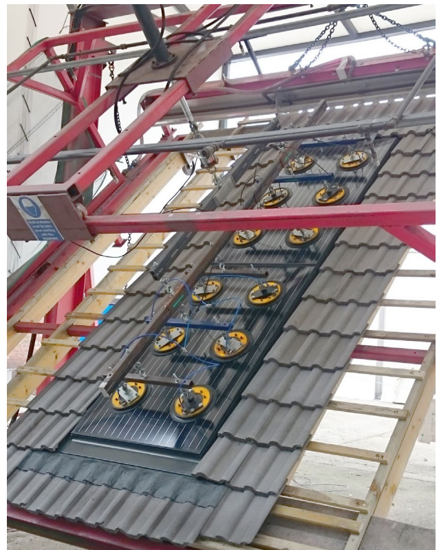
Clearline Fusion achieved the highest possible wind resistance during testing for MCS012
